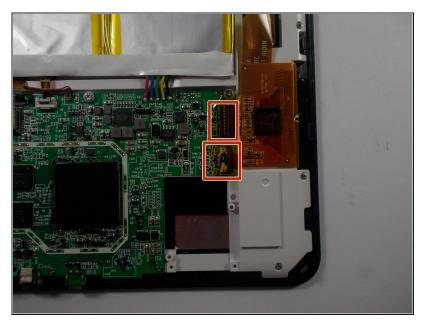
• Peel off the tape covering the two connections labeled in red.
