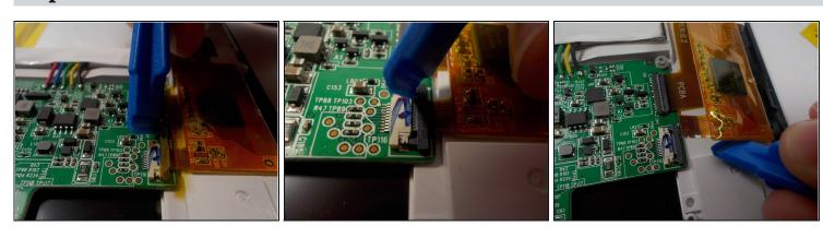
Remove the ribbon cable by lifting up on the connection with a plastic opening tool and pulling out the ribbon cable.
