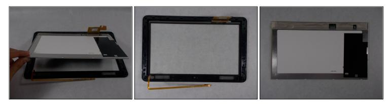
• The screen is now free. Lift the screen out of the glass panel. The screen can now be replaced.
