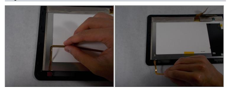
• Peel back the ribbon cable resting on the screen.
