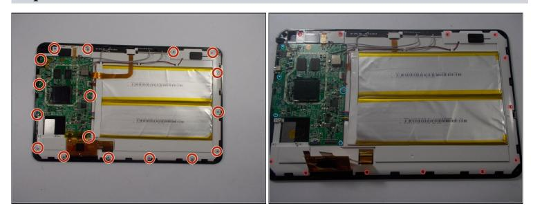
• Use a Phillips #0 screwdriver to unscrew the 17 screws labeled in red.
