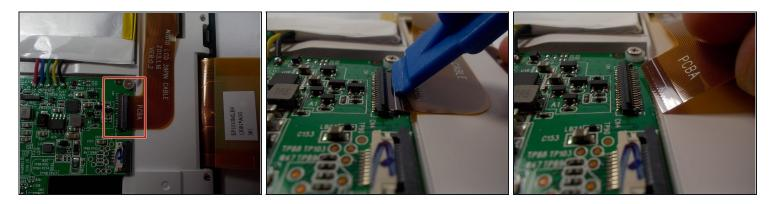
Remove the ribbon cable by lifting up on the connection with a plastic opening tool and pulling out the ribbon cable.
