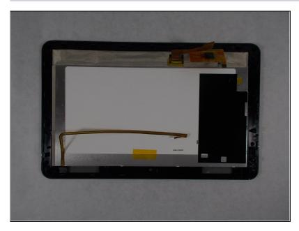
With the screws and white plastic cover removed, the screen and glass panel is exposed.
