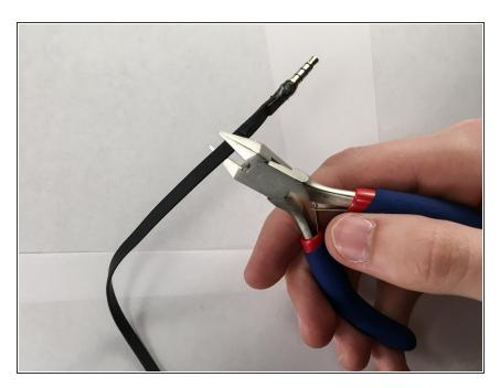
Cut the headphone cable near the old headphone jack. Leave some cable attached to the jack.
