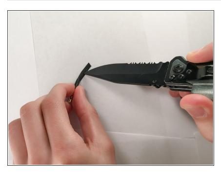
Cut open the outer insulation of the cable connected to the old jack to expose the internal wires.
