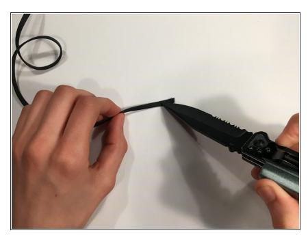
Cut away the insulation on the wire connected to the headphones.
