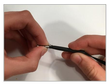
Slide the shrink tubing back over the base of the jack, covering the soldered connections.
