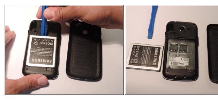
Once rear cover is off use small pastic spudger to lift battery out of the phone
