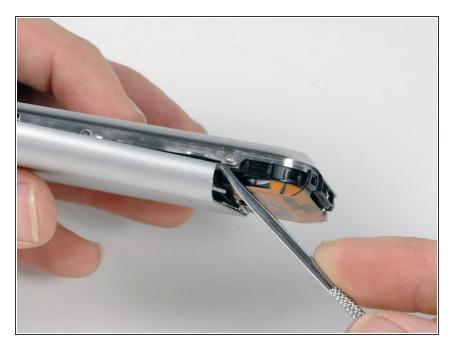
Pry up the rear panel by pulling the dental pick counterclockwise in a quick motion. Apply force perpendicular to the plane of the display assembly. You may be afraid to go fast, but going slowly is more likely to bend the case.
