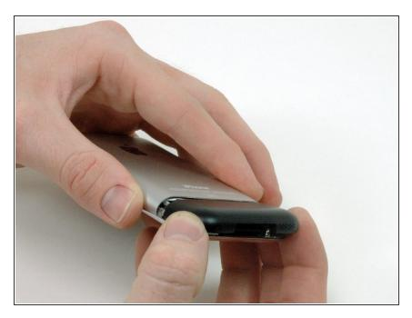
Grasp the antenna cover on either side and slide it up and away from the iPhone. This requires some force. If it does not come free, ensure that the antenna cover is lifted up enough to free the catches.
