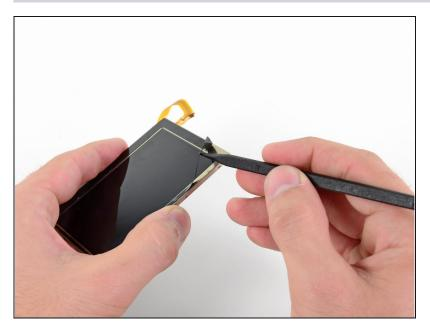
A strip of black adhesive tape holds the upper LCD to the display bezel. Use the tip of a spudger to remove the tape from the LCD housing.
