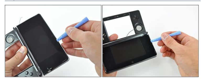
Continue prying the remaining sides of the front panel by sliding the plastic opening tool down each edge.
