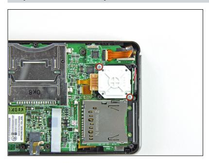
Remove the two 7.7 mm Phillips screws securing the back of the Circle Pad to the motherboard.
