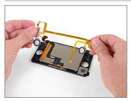
Remove the speaker assembly from the rest of the display assembly.
