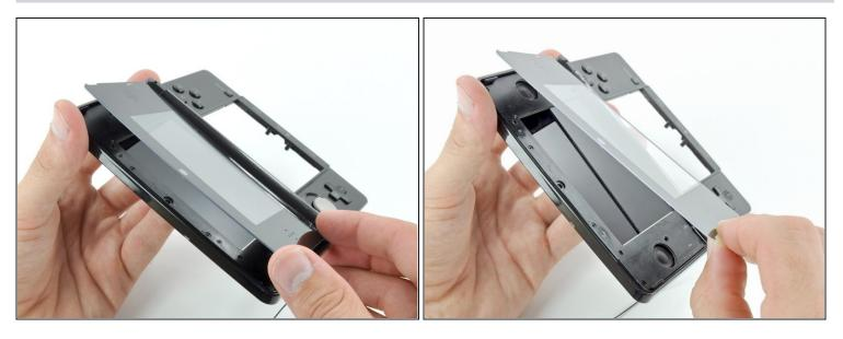
With all of the sides free, lift the upper display front panel off the display bezel.
