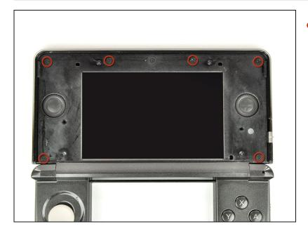
Remove the six 3.6 mm Phillips screws securing the rear display bezel to the front display bezel.
