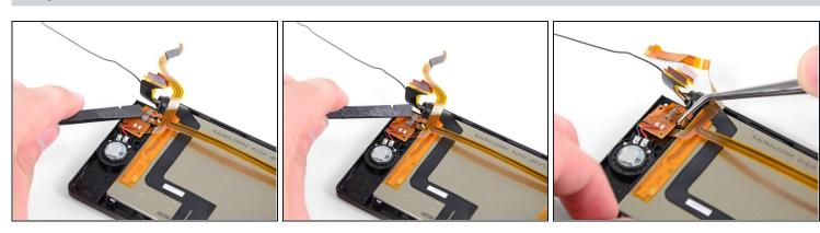
• Use the flat end of a spudger or your fingernail to flip up the retaining flaps on the parallax barrier ribbon cable ZIF sockets.
