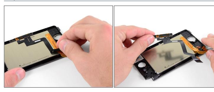
Peel the camera ribbon cable off the back of the upper LCD.
