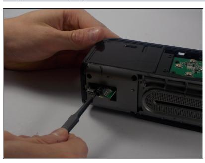
Locate the slit on the back of the device and the board will be located there. Remove board from slit by using tweezers.
