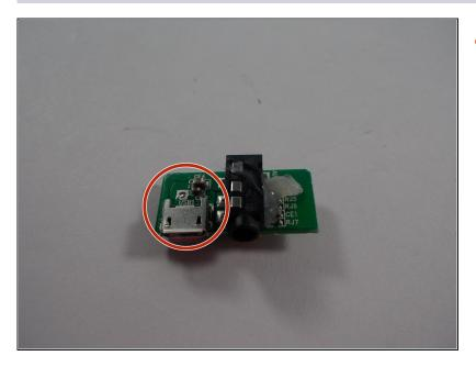
Once board is removed, locate silver component on the board. This is the charging port.
