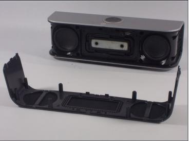
• To remove the front grate of the speaker grab a metal spudger and go to the back corner of the device where the front panel curves around the device. Insert the spudger and ply apart the corner until clips release from panel. Repeat for the other side of the grate. When all clips are released pull grate off from the front of device
