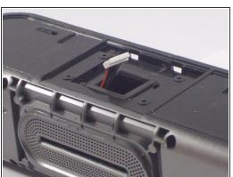
Using the nylon spudger, carefully remove the board from its socket. Next detach the wires from the chip to remove the board. After board is removed replace buttons.
