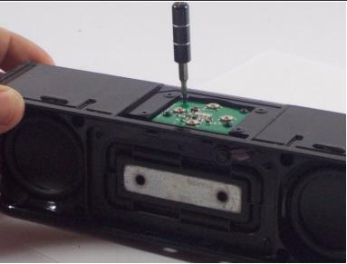
Locate the four, 6mm screws on the board on top of the device. Unscrew them with the PH0 bit on the screwdriver so that the board may be removed.
