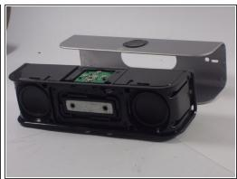
Grab two metal spudgers and insert one into the slit underneath the silver plating on the top of the device. Pry upward with the spudger until you unhook the two locks on the top. Repeat same step for the bottom of the device. When all four tabs are released, slide device out of the casing
