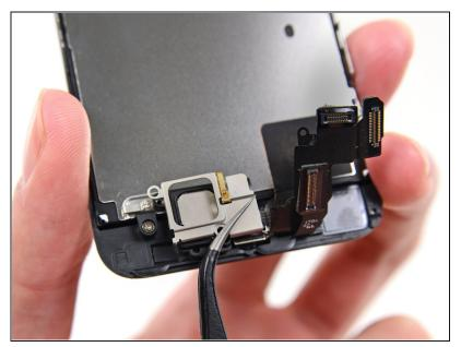
• Remove the bracket from the display.
