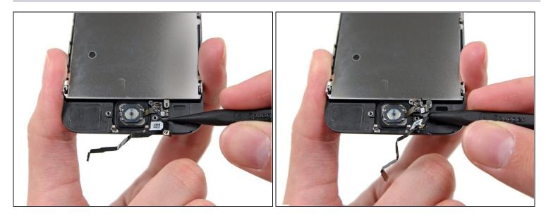
• Wedge the the tip of a spudger underneath the home button cable assembly.
