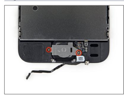
Remove the two 1.4 mm Phillips #000 screws from the home button bracket.
