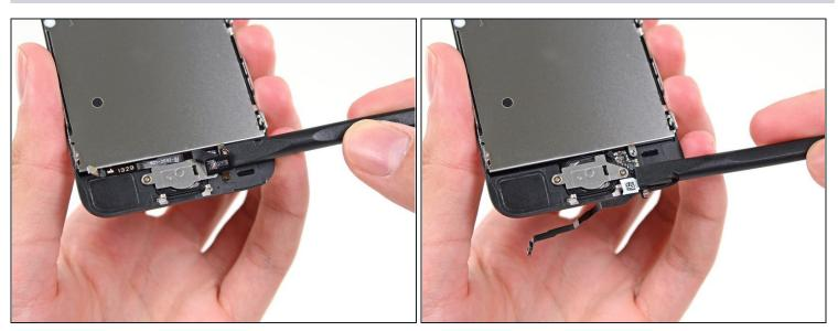
• Fold the home button cable down, out of the way of the home button bracket.
