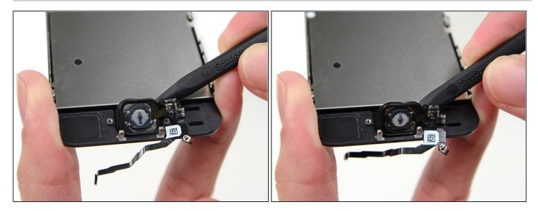
• Peel the home button the rest of the way off of the display by prying gently with a spudger.
