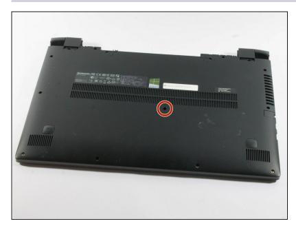
• Remove the one (40 mm) screw in the middle of the Flex 15.
