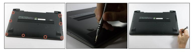
• Working your way around the outer edges of the Flex 15, remove the 8 (30 mm) outer screws.
