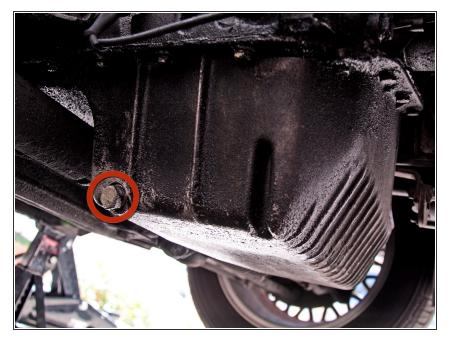
Locate the oil pan drain plug. It will be located on the passenger side of the oil pan nearest the center of the car.
