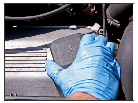
Twist the oil filler cap 1/4 turn counter-clockwise and remove it from the valve cover.
