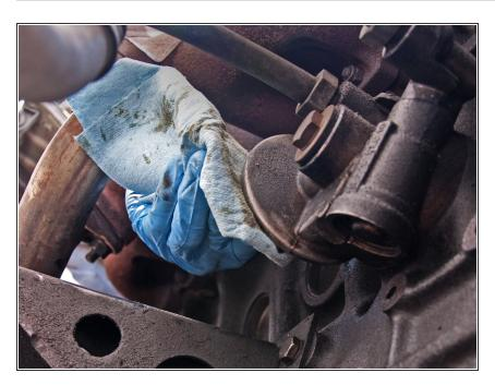
Use a clean paper towel to gently wipe the sealing surface on the oil filter housing.
