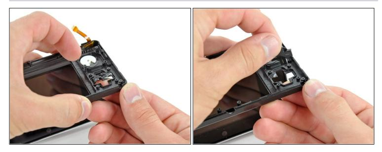
(i) Open the 3DS and orient it so that the bottoms of the buttons are facing upward.
