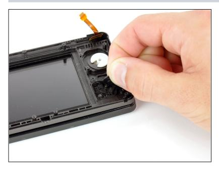
• Peel the black silicone cover off the back of the D-pad.
