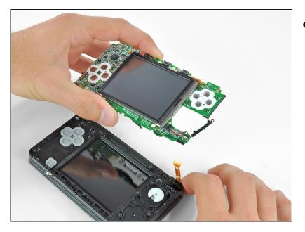
• Remove the motherboard assembly from the rest of the device.
