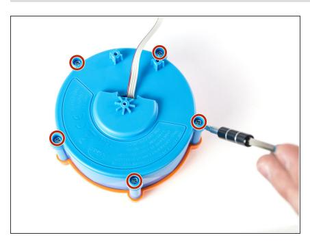
Loosen and remove the five 15 mm screws using a Phillips #2 screwdriver.
