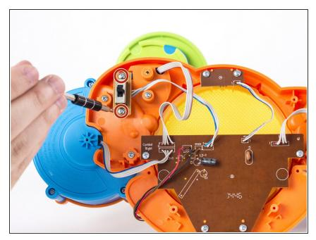
Loosen and remove the two 8 mm screws using a Phillips #00 screwdriver.
