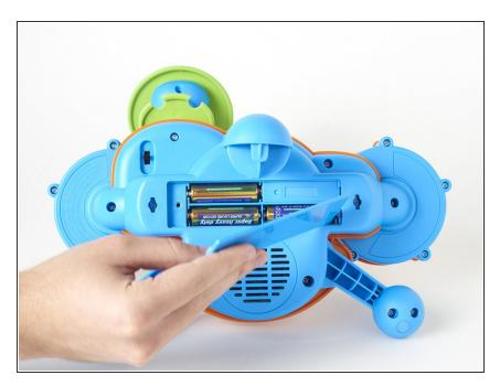
Using your fingers, pry open and remove the back battery panel.
