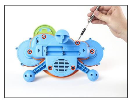
Using a Phillips #2 screwdriver, loosen and remove the six 14 mm screws.
