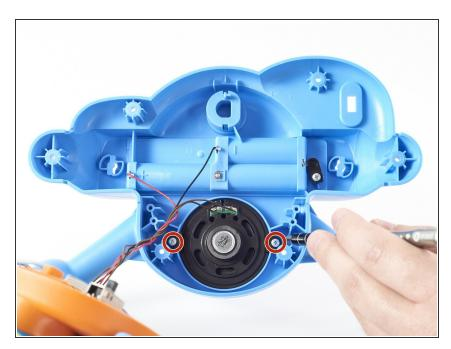
Loosen and remove the two 10mm screws using a Phillips #00 screwdriver.
