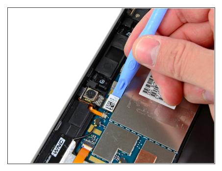
Use a plastic opening tool to pry the camera connector up and out of its socket on the motherboard.
