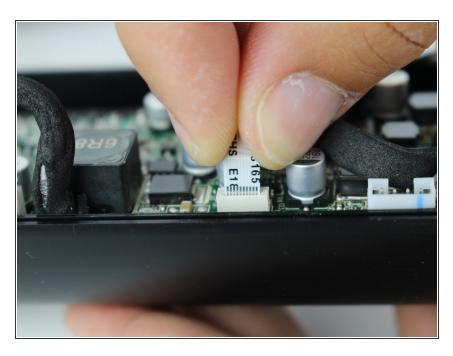
Carefully remove the cable connecting the control chip to the motherboard.
