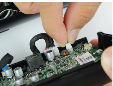
Use the black spudger to disconnect the auxiliary wire from its socket.
