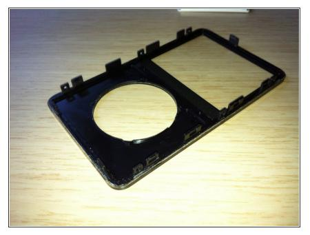
Use this photo of the OPENED iPod for the reference, in order to locate the areas where the retaining clips are - 4 per side, one on top and two at the bottom. It should save you a lot of frustration and help avoid scratching the plastic cover.
