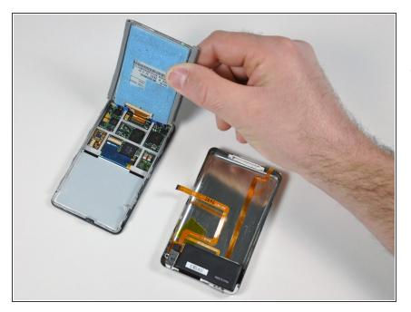
The front and back of the iPod should now be completely separated.
