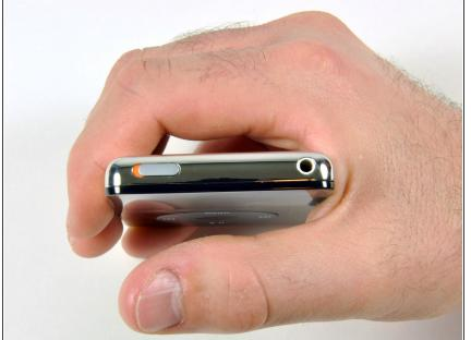
(i) Before opening your iPod, ensure that the hold switch is in the locked position. The slider should be all the way to the right if your iPod is facing you.
