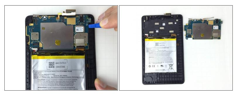
• Position the iFixit Opening Tool beneath the motherboard and pull upwards to remove the motherboard from its case.
