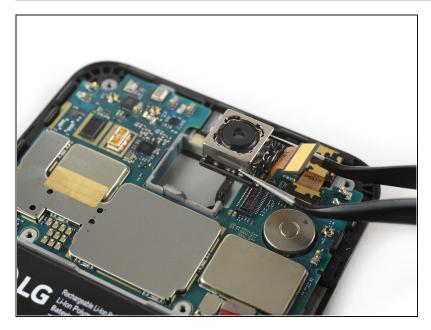
Use a pair of <u>tweezers</u> to remove the rear facing-camera.
