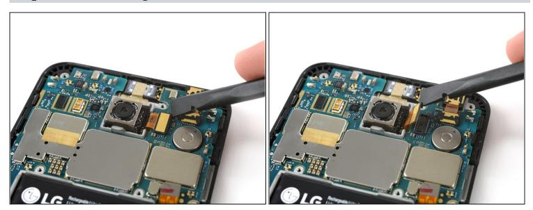
• Use the flat end of a spudger to pry up the rear facing camera's flex connector.
