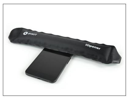
• <u>Use an iOpener</u> to loosen the adhesive beneath the rear facing camera. Place the iOpener across the top part of the phone for about 30 seconds.
