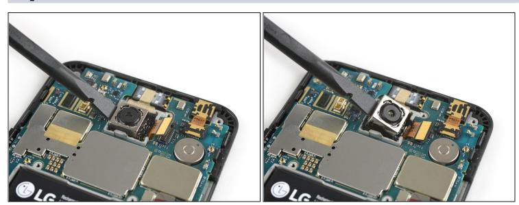
• Apply the flat end of a spudger to the left side of the rear-facing camera and carefully lever it out of its recess.
