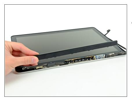
Remove the clutch cover from the display.
