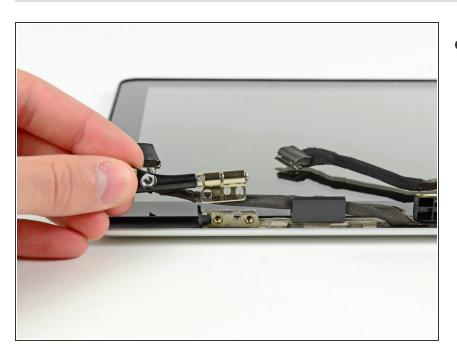
Remove the left clutch hinge from the display.
