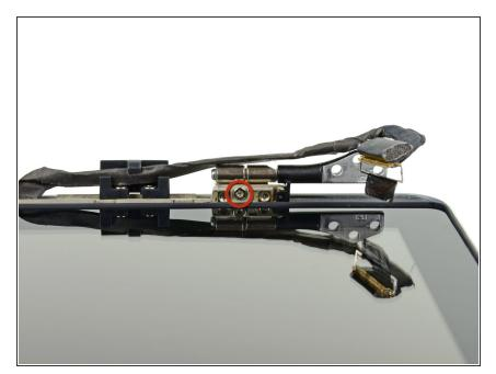
Remove the single 5.2 mm T6 Torx screw securing the left clutch hinge nearest the display glass.
