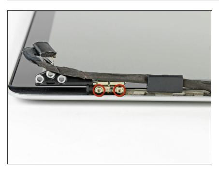
Remove the remaining two 5.2 mm
