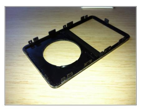
Use this photo of the OPENED iPod for the reference, in order to locate the areas where the retaining clips are - 4 per side, one on top and two at the bottom. It should save you a lot of frustration and help avoid scratching the plastic cover.
