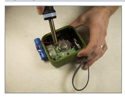
Using a soldering iron, heat up and remove the positive and negative wire contacts from the motherboard.
