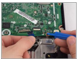
Use a plastic opening tool to carefully lift the white hinge up on the touchpad cable connector, and gently remove the cable from the motherboard.
