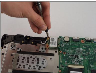
Remove one 6.2 mm Phillips #1 screw from the wireless chip on the left side of the motherboard.
