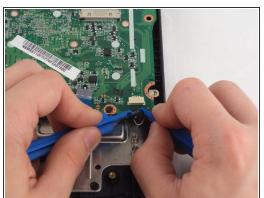
Use two plastic opening tools to grip each side of the connector for the speaker cable and gently pull the cable from the motherboard.
