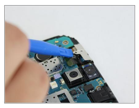
Remove metal cover with plastic opening tool.
