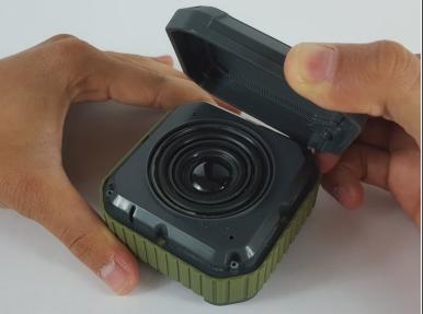
Carefully remove the front case by gently pulling it from the body of the device.
