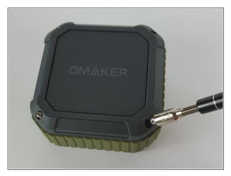
Use a magnet to remove the screws after unscrewing them and place them aside.
