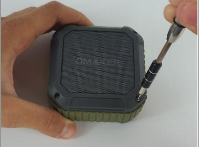
Use a T6 Torx Screwdriver to remove the four screws from the front of the device.
