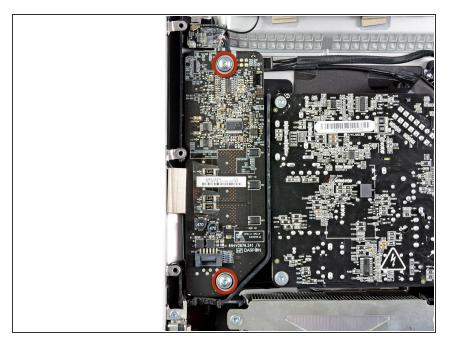
Remove the two 9 mm T10 Torx screws securing the LED driver board to the outer case.
