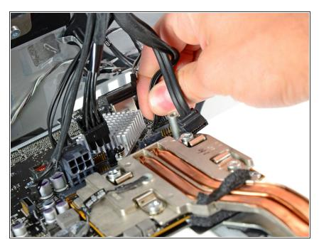
Pull the hard drive power cable connector out of its socket on the logic board.
