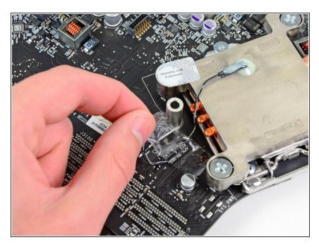
Peel the piece of tape covering the heat sink thermal sensor cable up off the logic board.
