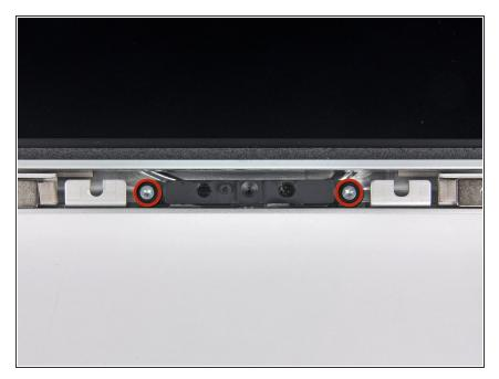
Remove the two 5.2 mm shouldered T10 Torx screws securing the camera board to the outer case.
