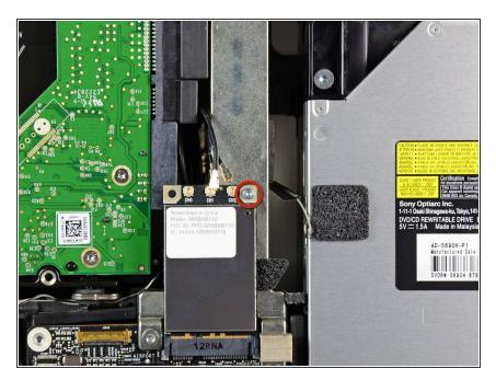
Remove the single 5.3 mm T6 Torx screw securing the AirPort card to its socket.
