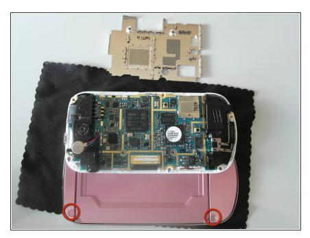
• Remove the EMI shield and remove the screws for the screen under the plastic stickers here.
