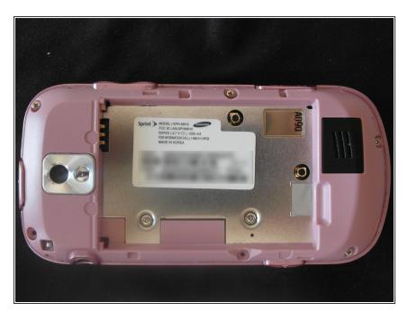
• Remove battery cover, battery and memory card.
