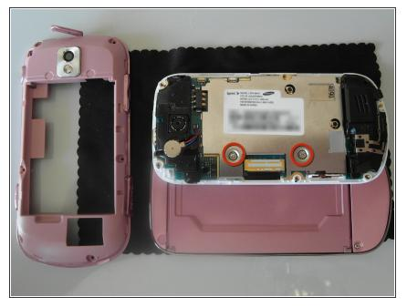
• Once the case is removed, remove the screws from the EMI shield.
