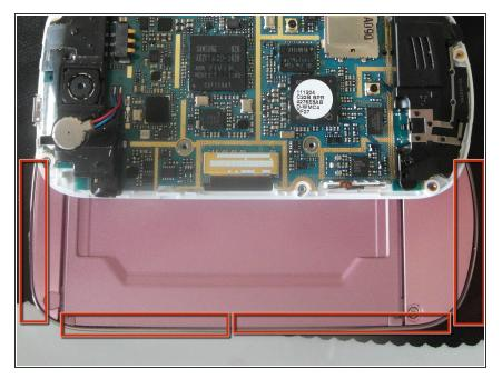
Insert your opening tool here to gently pry open the screen bezel.
