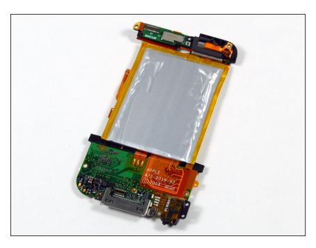
The other side of the wireless circuitry, battery, and logic board.
