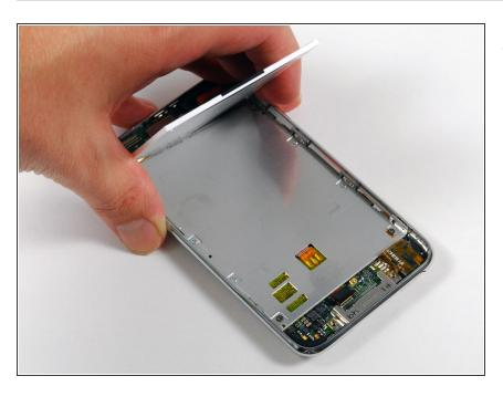
There are no screws securing the LCD. Instead, it's held in place with a little double-sided tape.
