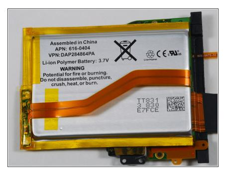
The battery. 3.7 V Lithium-ion polymer, as expected. Apple part number 616-0404. No word yet on the mAh rating.
