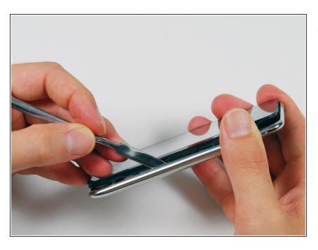
Removing the glass display and touch screen digitizer combo.
