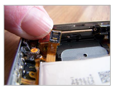
Headphone jack connector 5, the vibration motor, and the volume switch show some light corrosion.
