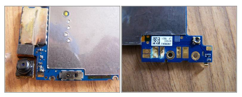
Rear of motherboard showing some signs of corrosion to battery contacts.
