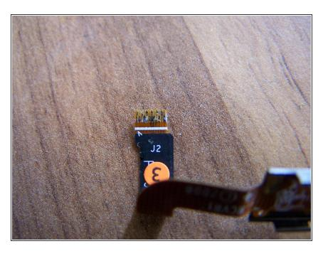
Closer inspection of proximity sensor/earpiece flex reveals more corrosion damage.
