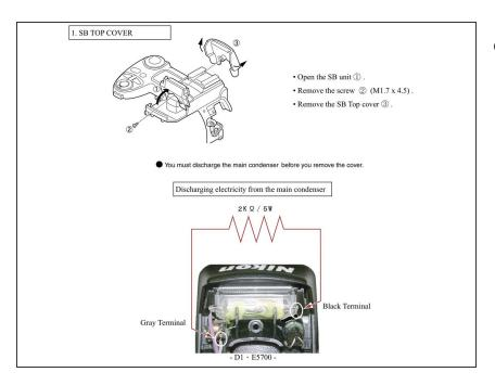
In order to pull the top panel without removing the flash unit. You must remove the flash top cover, taking away the screw under the bulb (see image). then gently remove the plastic top cover. IMPORTANT: discharge the condenser as soon as possible (the flash wires are now exposed, and dangerous).
