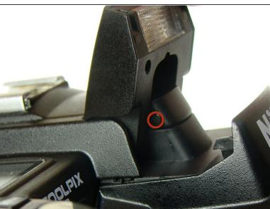
Remove the Phillips screws on both sides of the flash bulb mount.
