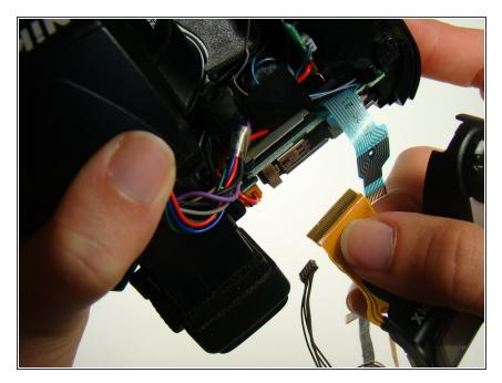
Unplug the orange ribbon and the other wires and finish carefully removing the top panel.
