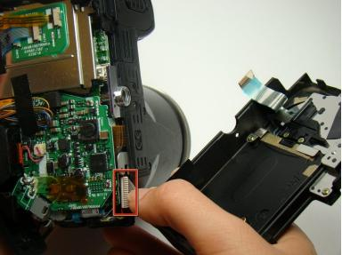
Now gently unplug the two wires at the bottom of the panel.
