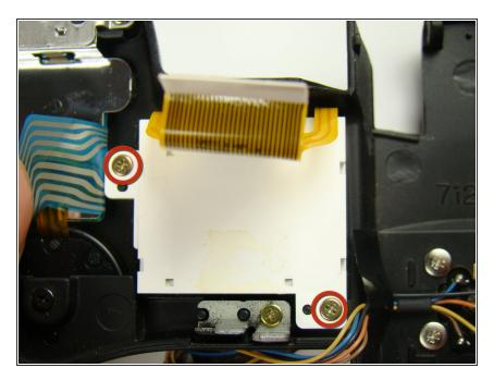
Remove the two gold Phillips screws (3.9 mm) holding the white panel down.
