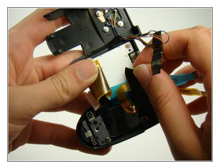
Remove the black tape holding the wires to the cover.
