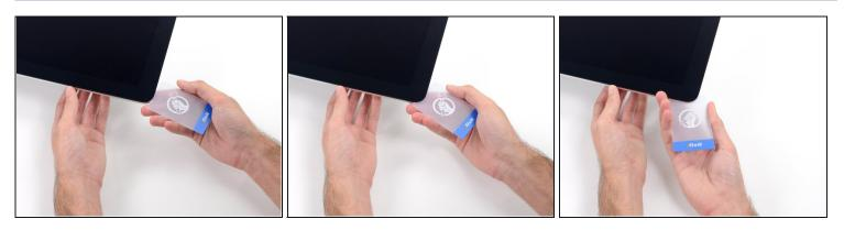
• Insert a second plastic card into the gap between the display and frame near the top left corner of the iMac.
