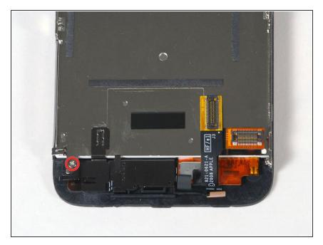
Remove the single Phillips #00 screw from the corner of the display assembly.
