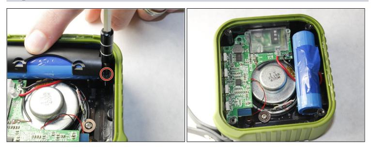
A Remove the two Phillips screws which hold its battery casing on the housing using a PH00 Phillips screwdriver.
