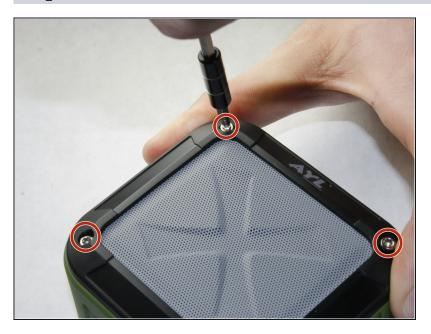
Unscrew the four hex screws on the top of the device using a 2.5mm hex screwdriver.
