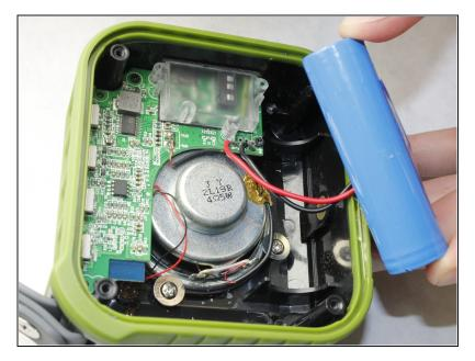
• Using a soldering iron, heat up and remove both the positive and negative battery contacts from the motherboard.
