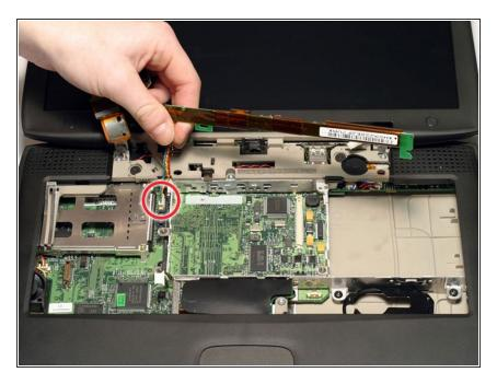
Disconnect the inverter plug, pulling directly up from the logic board.
