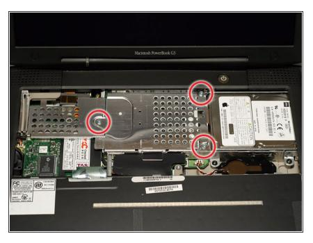
Remove the three silver Phillips screws that attach the heat shield to the internal metal framework.
