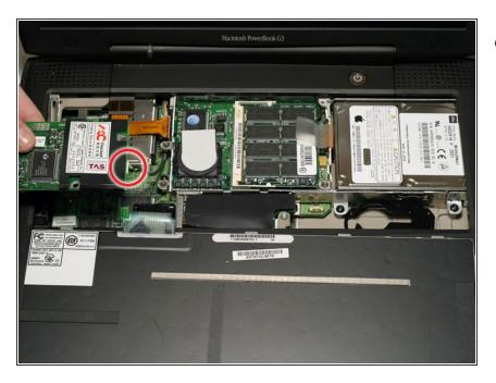
Disconnect the cable from the right side of the modem.
