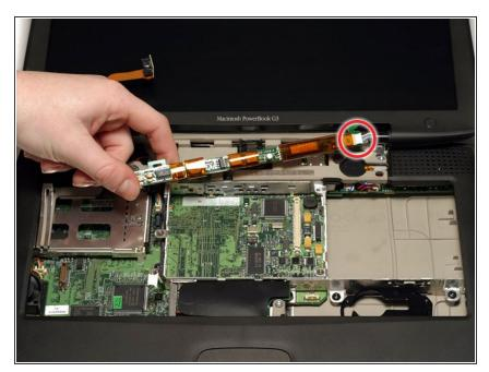
Disconnect the white inverter cable connector from the right end of the board.
