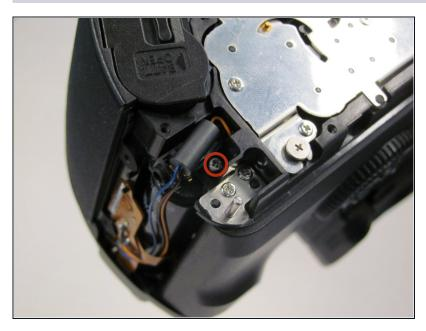
• Remove one 4.8 mm silver screw securing Remote Control Socket to camera.
