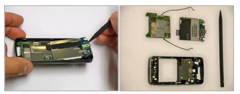
• Gently lift the motherboard up using a nylon spudger.
