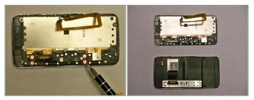
• Remove the 4 screws circled in red using a 00 Phillips-head screwdriver.
