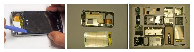
• With the front keyboard removed, gently lift the screen up with a plastic opener tool and remove it .
