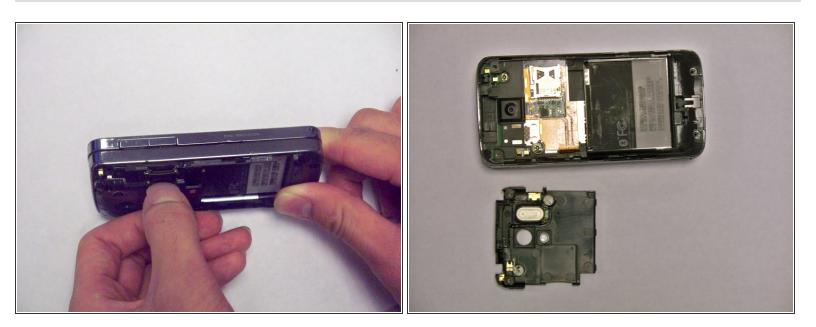
• Lift the plastic cover near the memory card slot.
