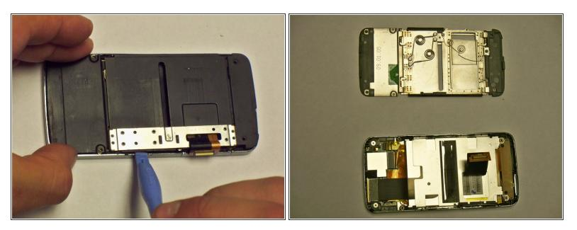
• Start by lifting the back plate of the screen by using yours finger or a plastic opener tool.
