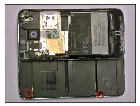
• Remove the two Phillips #00 screws from the backside of the screen.
