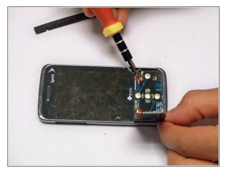
Lift the front keyboard by removing the screws with a 00 Phillips-head screwdriver.
