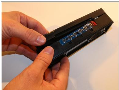
Pull apart the two faces to separate the back panel from the front face plate.
