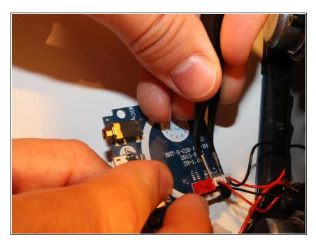
Use the tweezers to push down on the two safety prongs on the plastic switch. Then Disconnect the two Speaker plug connections by hand (Two Smaller Plugs)
