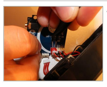
Use the tweezers to push down on the safety prongs on the plastic switch. Then Disconnect the Power Wire plug by hand (Red medium),
