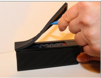
Using Blue Plastic opening tool pry the top rubber cover, then using the same tool remove the bottom panel
