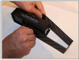
There are four prongs on the grill in the corners, closest to the power button switch. Use the plastic opening tool to release all four prongs from the panel, and then slide the plastic opening tool along the edge of the grill to allow it to easily slide off.
