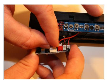
Disconnect the Button Panel plug (Largest of the Plugs, it can be traced back to the button panel easily)
