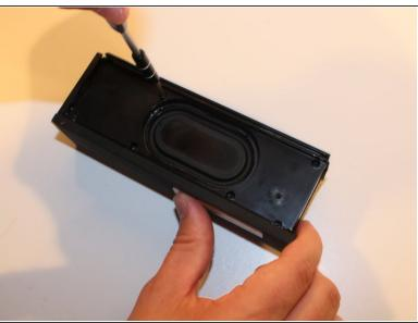
On the back panel (Opposite to the side containing the two speakers), Use the Philips head PH1 to remove all 7 screws (Screws: Head PH1, Length 7cm).
