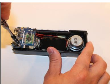
Remove the single screw holding the motherboard to the front panel (Screw: Head PH1, Size .5 cm)
