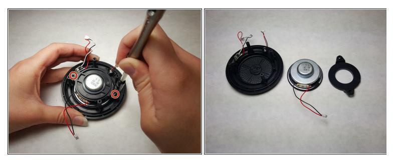
After the speaker is detached, remove the two 8.5mm screws that hold the speaker to the front panel with a Phillips #1 screwdriver.
