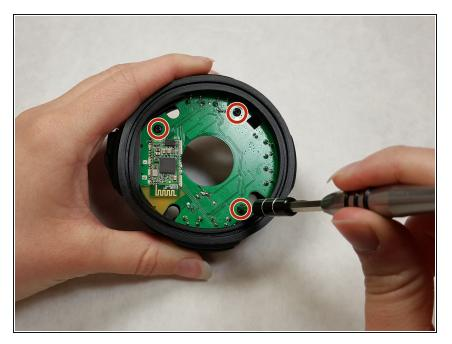
From the back of the motherboard, unscrew the three phillips head screws holding the motherboard in place.
