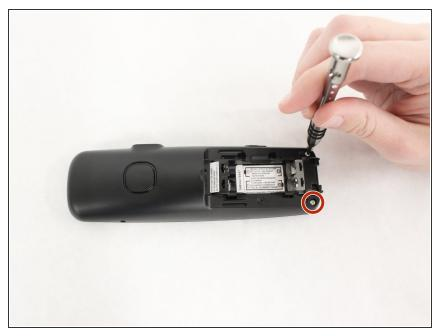
Remove the two screws behind the battery panel by using a Philips size #00 screwdriver.
