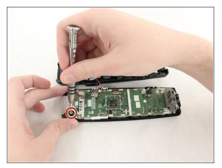
Using the same screwdriver as before, remove the Philips size #00 screw holding the motherboard in place.
