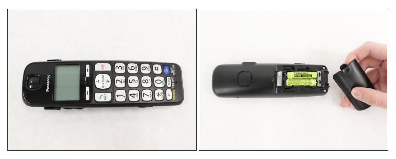
• Flip the handset over to expose the back panel, and slide the panel out to remove.
