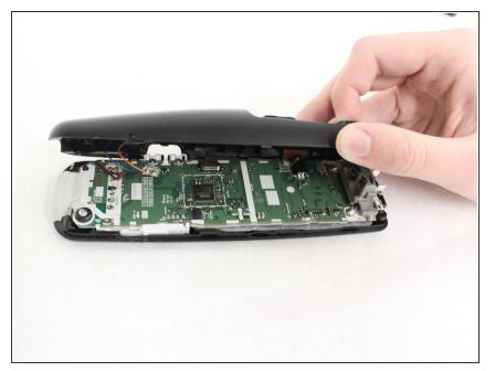
Once the back has been separated from the rest of the device, carefully place it to the side. Be careful not to completely remove it, however, as there are wires connecting the back to the handset.
