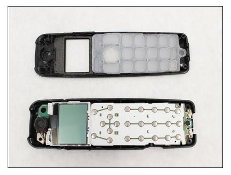
• With the screw removed, the front panel assembly can be separated from the rest of the device.
