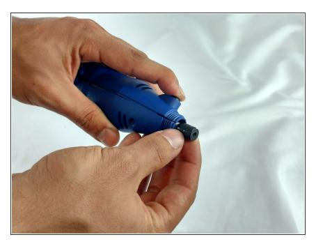
• While pressing the spindle lock button, unscrew the collet nut and remove it along with the brass collet.
