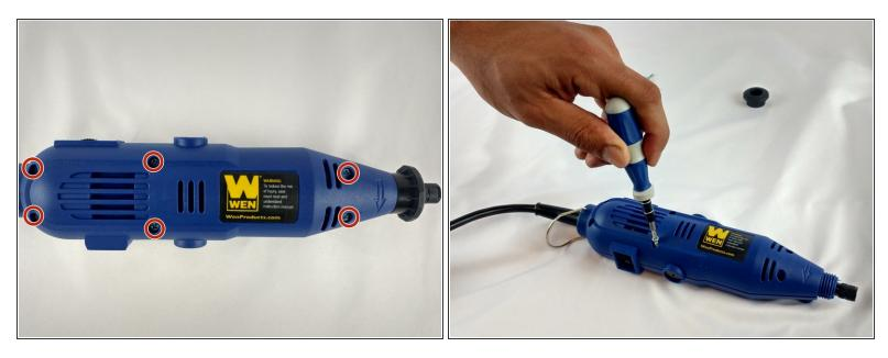
Unscrew the six 8mm PH2 screws.
