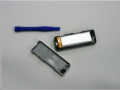
Carefully pry the backing of the device away from front of the device. This can be done by wedging the opening tool in the crack where the two sides of the device cover meet.
