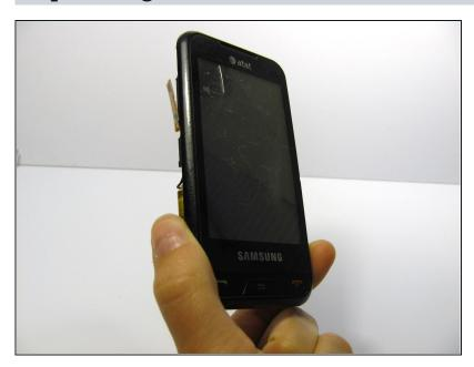
Flip phone over so you are looking at the front screen of the phone. (The back is already taken off and parts removed)
