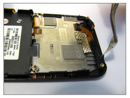
• Peel up the black tape on the bottom of the back case.
