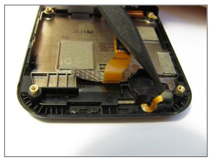
• Pop the microphone up and out of its small housing.
