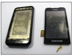
• Use a small tool to pry the digitizer and screen (together) from the frame of the phone. This may take some time and careful work because it is glued down to the frame.
