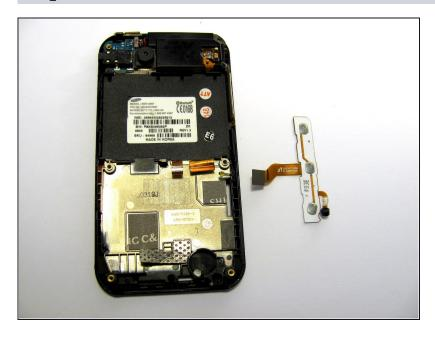
The front button board should slide out. At this time you can replace the button/microphone component.
