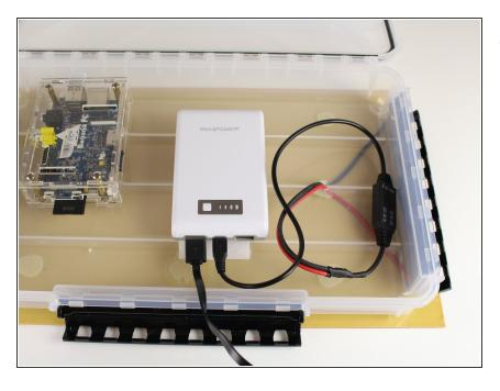
Place the battery pack down on the hook Velcro inside the box.
