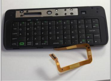
• Pry the keyboard away from the screen. Open on the side containing the keyboard ribbon.
