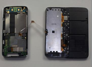
Insert your spudger along the slit between the keyboard and the external casing. Pry open as shown.
