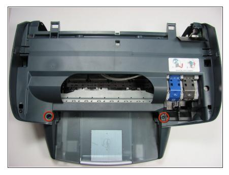
Remove the two black screws closest to the printer tray.
